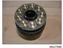
(21) Assemble rotary block kit into casing (1).
