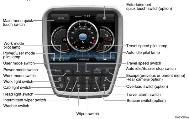
When some of the switches are selected, the pilot lamps are displayed on the LCD. Refer to the page 5-61 for details.
