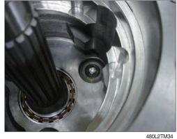
(11) Disassemble pivot (14)-2EA from casing (1).
