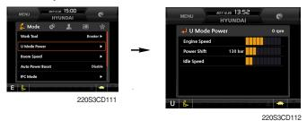
Engine high idle rpm, auto idle rpm and pump torque (power shift) can be modulated and memorized separately in U-mode.
